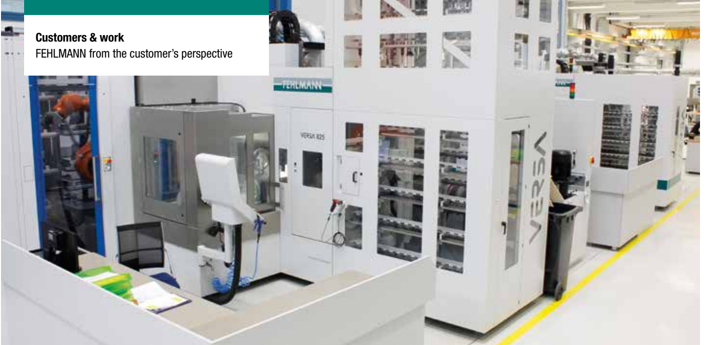
The FEHLMANN VERSA 825 and the rack magazine for 346 tools are core components of the automation solution at Test-Fuchs.
