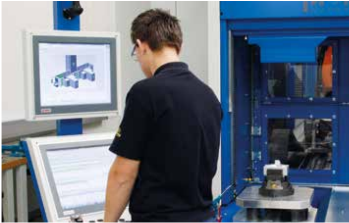
The automation cell with rail system, loading and unloading station, robot and host computer was supplied by Promot Automation.
