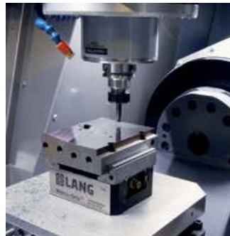
The linear drives not only achieve faster traversing movements, but also allow more precise imaging in corner areas. Tolerances of 1/100 mm are thus achieved reliably and permanently.
