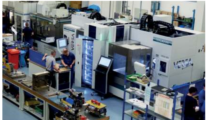
The decisive criteria for the machining cell were compactness and the operator's ability to always have an overview of both machines.
