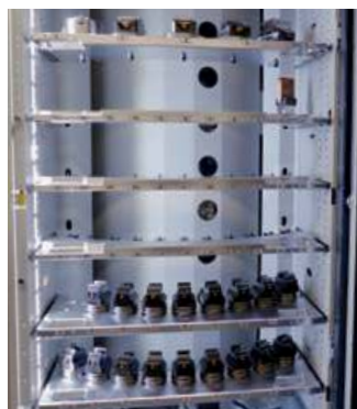
A small challenge for Fehlmann: 320 x 320 UPC pallets, ITS 85 and 148 as well as electrode holders are used.
