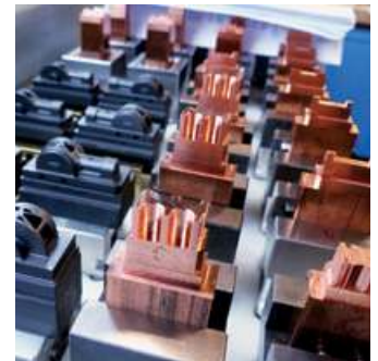
The two machining centers are utilized 30 percent with the milling of copper electrodes. Independently of this, WESKO also manufactures graphite electrodes, but on a different machine.
