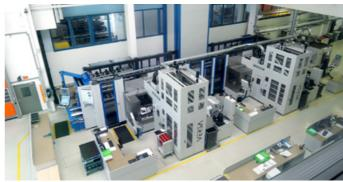
Linear automation solution consisting of two VERSA 825 with rack magazine
