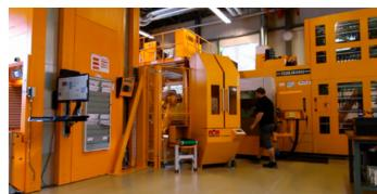
Articulated-arm robot and Goodj automation system on a VERSA 825 with rack magazine for 346 tools
