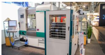
Articulated-arm robot FMB for handling blanks on a PICOMAX 75
