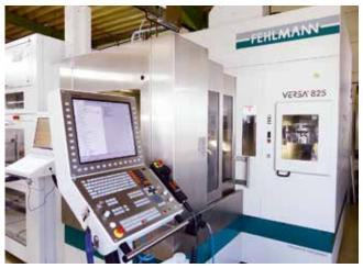
1 Expect the unexpected: instead of a single machine for 5-axis machining, a Versa 825 5-axis simultaneous machining centre from Fehlmann complete with Erowa automation now carries out challenging tasks at G. & K. Schön (Photo: Fehlmann)
