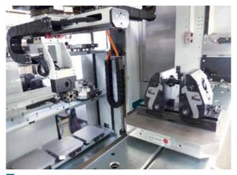
2 The Erowa robot Leonardo carries in its standard version up to 24 UPC palettes (320 mm × 320 mm). The production unit is primarily used to manufacture cages made from case-hardening steel for roller burnishing tools (Photo: Fehlmann)
